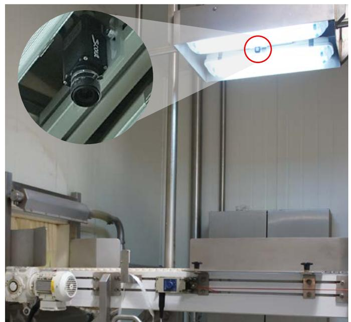
Basler's scout GigE camera is installed below a light source above the conveyor and captures the artwork on the powder bags.
