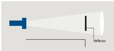
Teach-in for a two-way reflective barrier with a firmly fitted reflector
