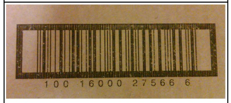
The effectiveness of an automated data collection system can be hampered by low quality input. Shipper barcodes printed on brown corrugated cases have low contrast scores in the best of circumstances. As print nozzles become clogged or there are inconsistencies in line speeds the quality of the code degrades, making it impossible for most barcode scanners to reliably read them.
