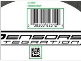
The CRIS has verification options using SICK laser scanners and vision cameras for UPC and data matrix codes at speeds of up to 1200 inspections per minute.
