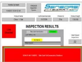
The multi-patented design assumes every product should be rejected until positively verified by the system to ensure product safety and accuracy. Faults in any part of the line will prevent products from continuing past the inspection point.
