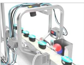
Our reject system tracks product pass signals as they pass the inspection point and uses our patented algorithm to accurately reject products even with continuously varied line speeds.
