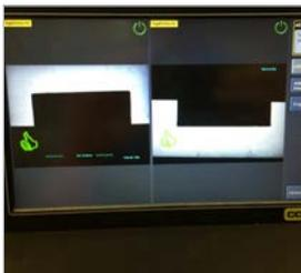
Customized algorithms for vision allow detection of open flaps on containers early in the production process.
