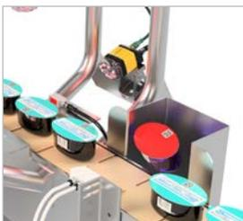
Our reject system tracks product pass signals as they pass the inspection point and uses our patented algorithm to accurately reject products even with continuously varied line speeds.
