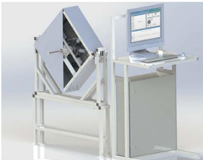
*Machine vision system for continuous control of diameter and ovality of products with cylindrical shape.*
